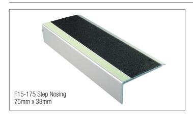
The F15-175 Step Nosing is designed to ensure visibility of steps in escape routes for compliance with NCC E4P1 Visibility in an Emergency requirements as a Performance Solution. The step nosing will be effective in all light conditions including during failure of the main lighting.
