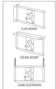
Ecoglo passive photoluminescent (PL) signs are designed to provide identification of exits. The signs will be clearly visible to occupants, and operate in the event of power failure to the main lighting system.
